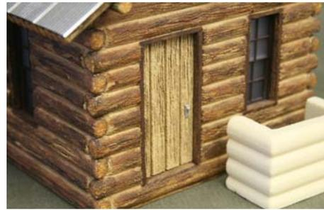
Our Wood Plank, Large or Small Board & Bat, and Log patterns have the joints between boards and logs already planed into the Precision Board. You can round edges of boards and logs as desired. Wood texture is added with wire brushes. Knot holes, splits in wood, etc., can be done with a Dremel®, dental tool or craft knife.
