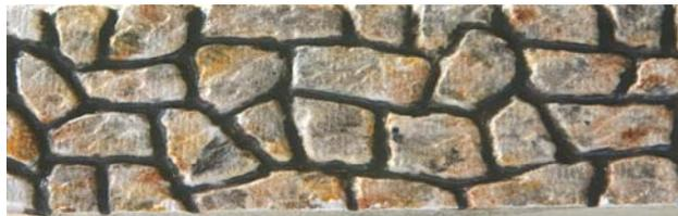
Smooth surface material can be carved or fabricated with any tools that can be used on wood. The range of possibilities is only limited by your imagination. You can create random stone, flagstone, fieldstone, random wood pieces, etc., etc.
